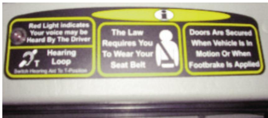
driver on the other side of a plastic screen gives me walking directions, I hear clearly, because all London taxis have induction loops that broadcast the driver's voice to t-coil-equipped hearing aids. As I pay the driver, I can't resist asking where his microphone is. With a smile, he points to the built-in mini mic right next to the visor in front of his face.
